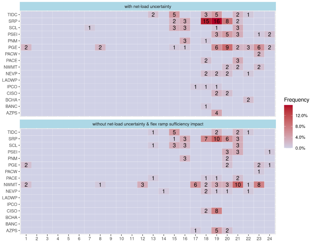
Figure 81: Daily Frequency of upward capacity test failures for all EIM BAAs with consideration of flex failures
