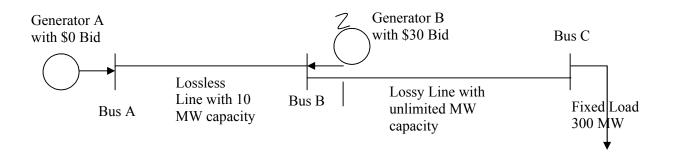
The MW solution is the same as example 1 with Generator A dispatched at 10MW and Generator B dispatched at 305MW.
