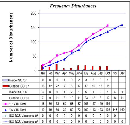
Frequency Disturbances are results of a sudden loss of load or generation. ISO DCS Violations are those losses of generation greater than 35% of our most severe single contingency (currently 399 MW), where the ACE is not recovered within 15 minutes. The DCS Violation Target Goal is not to exceed 2 ISO DCS violations, with the Stretch goal of zero violations for the calendar year. Our YTD results are on track to meet the Stretch objective to have zero DCS Violations for 2007.
