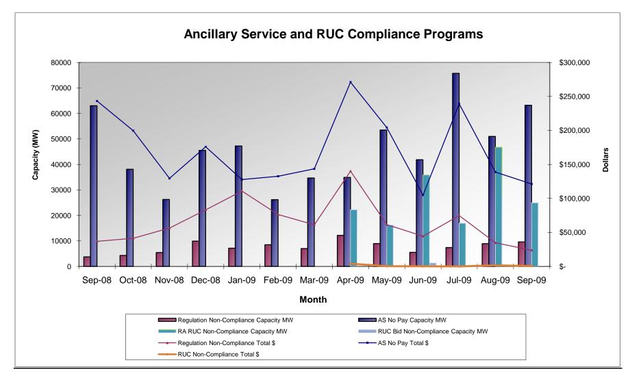
Ancillary Services and RUC Compliance Program: shows the monthly totals of non-compliant ancillary service capacity (MW) for twelve months and non-compliant RUC capacity (MW) beginning April 2009. Operations Support monitors suppliers of ancillary services and RUC to ensure that ancillary service and RUC capacity awarded in the ISO markets is available in real-time.
