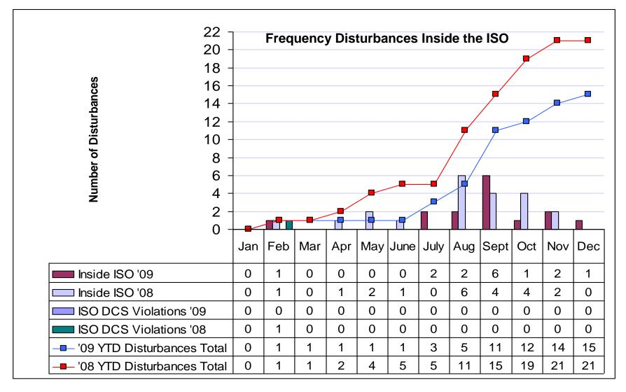
**NOTE:** This graph now depicts data for "Disturbances Inside ISO" for both '08 and '09 for appropriate comparison. **Frequency Disturbances** are results of a sudden loss of load or generation.
