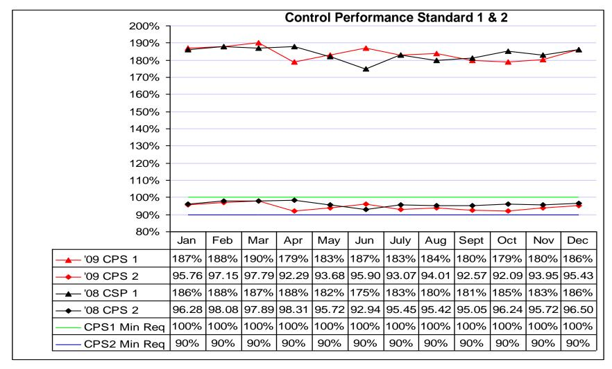
**CPS1** is a statistical measure of Area Control Error (ACE) variability. It measures ACE in combination with the interconnection frequency. The CPS1 formula was developed on a conformance scale, therefore values over 100% are not only desired, but also expected. **CPS2** is a statistical measure of ACE magnitude. It is designed to limit a Control Area's unscheduled (or inadvertent) power flows that could result from large ACE values.
