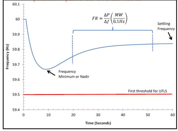
Accurate models of governors are needed to ensure compliance with the NERC Standard BAL-003
