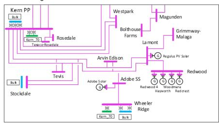
Figure 3.6-59 Kern PP-Tevis 115 kV LCR Sub-area
