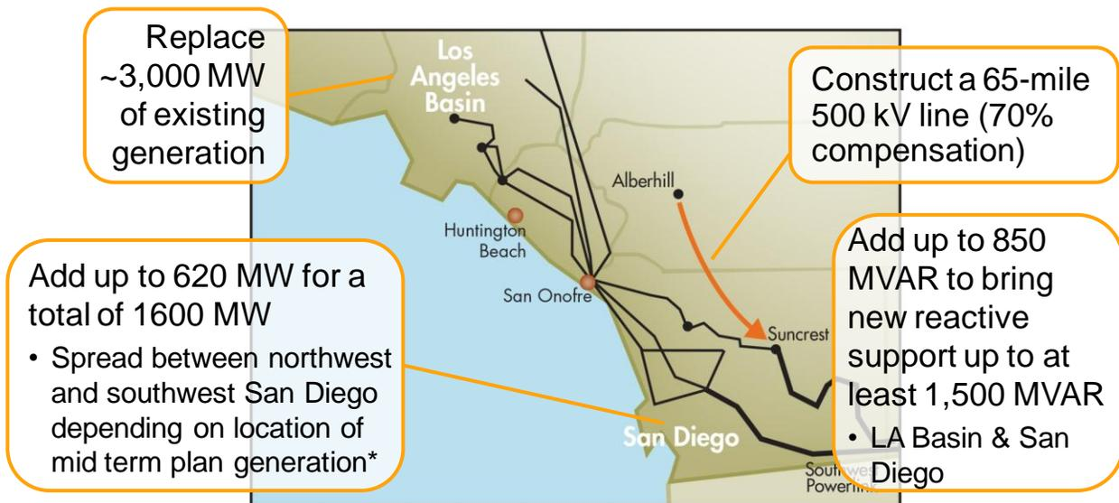
\*Approximately 700 MW of generation in San Diego can be displaced by additional reactive support, transformer upgrades and 66 kV transmission upgrades in the LA Basin and upgrading line series capacitors and additional transformer upgrades.
