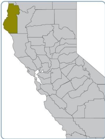
Humboldt's electric transmission system is composed of 60 kV and 115 kV transmission facilities. Electric supply to this area is provided primarily by generation at Humboldt Bay power plant and local qualifying facilities generation units. Additional electric supply is provided by transmission imports via two 100 mile, 115 kV circuits from the Cottonwood substation east of this area and one 80 mile 60 kV circuit from the Mendocino substation south of this area.
