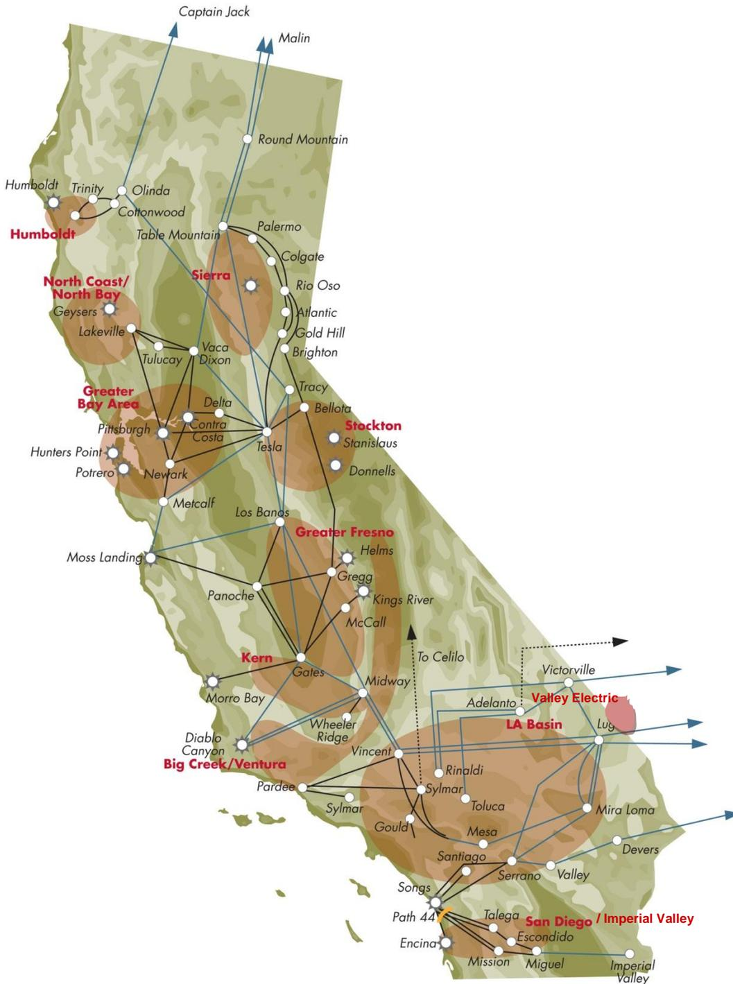
Each load pocket is unique and varies in its capacity requirements because of different system configuration. For example, the Humboldt area is a small pocket with total capacity requirements of approximately 200 MW. In contrast, the requirements of the Los Angeles Basin are approximately 10,000 MW. The short- and long-term LCR needs from this year's studies are shown in the table below.
