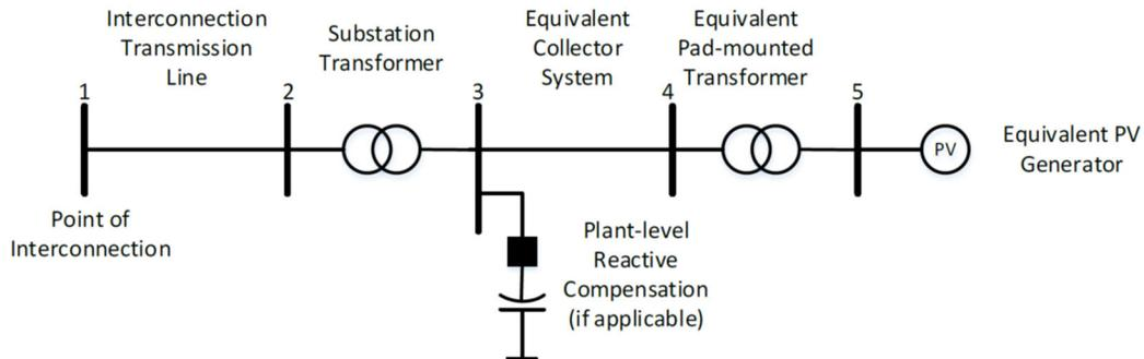
**Figure 2: Multiple-Generator Equivalent Power Flow Representation for a Solar PV Power Plant**
