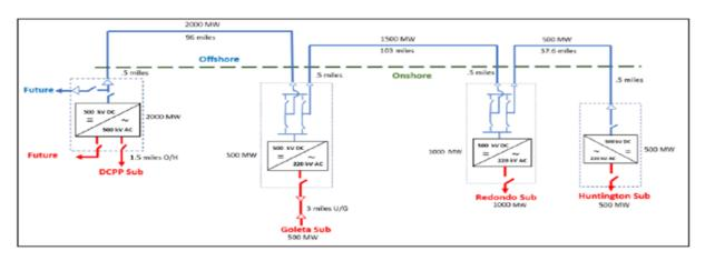
Figure 4.10-18: Proposed Pacific Transmission Expansion HVDC Project
