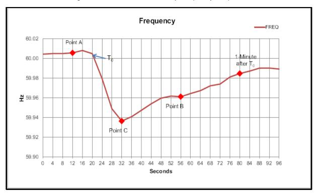
Figure 6.3-1: Illustration of Primary Frequency Response
