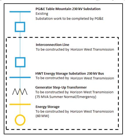
Figure 2.4-2. Table Mountain 230 kV Substation Energy Storage Project
