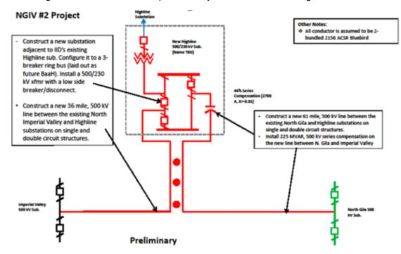
Figure 4.8-2: North Gila - Imperial Valley #2 500 kV Line Configuration
