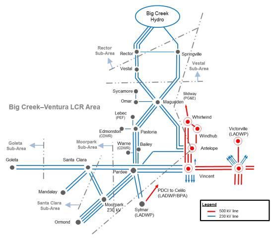
Figure 4.10-6: Big Creek-Ventura Area Transmission System
