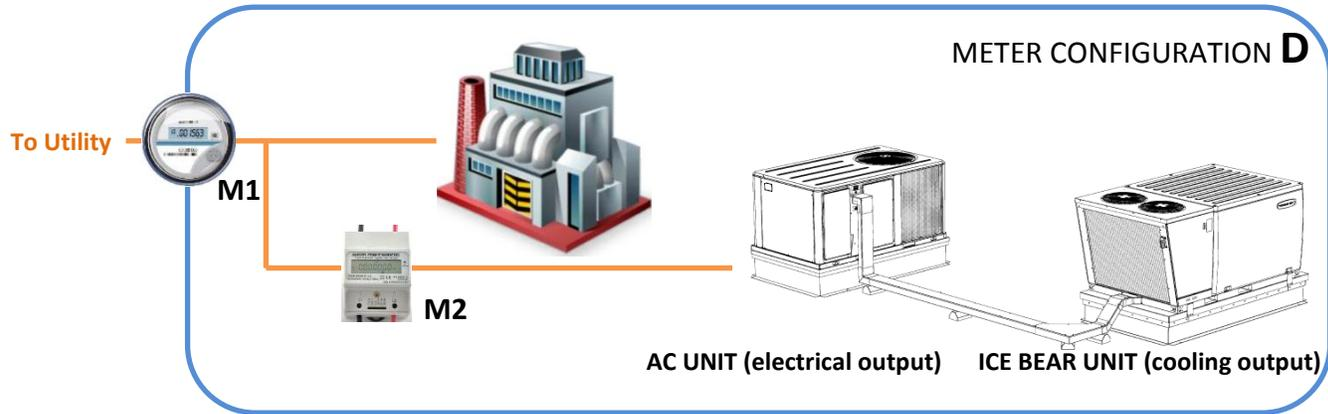
The current configuration for the Ice Bear is to connect directly to a commercial customer’s AC system. Each unit is equipped with internal performance data that can be converted to metering data, represented by M2. This simple M2 meter will not be sufficient to bid Dispatchable Load (DL) into the real-time market under current CAISO rules, but may be sufficient to bid Permanent Load Shifting (PLS) into the day-ahead market as described below in Use Case #2.
