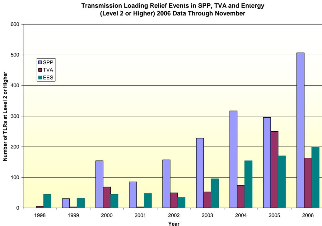
**Figure 4: Transmission Loading Relief Events for SPP, TVA and Entergy**
