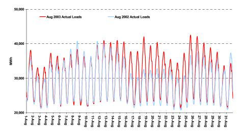
Figure 1b. Actual Load in the ISO Control Area for August: 2003 v. 2002
