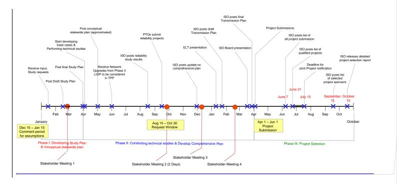
Figure 2-1: Overview of the scope and timelines of Phase 1-3 in the ISO Transmission Planning Process
