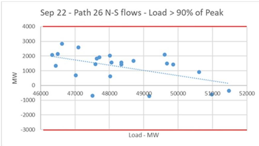
Graph 1: Path 26 loading levels during September 2022 periods when the load was above 90% of the peak.
