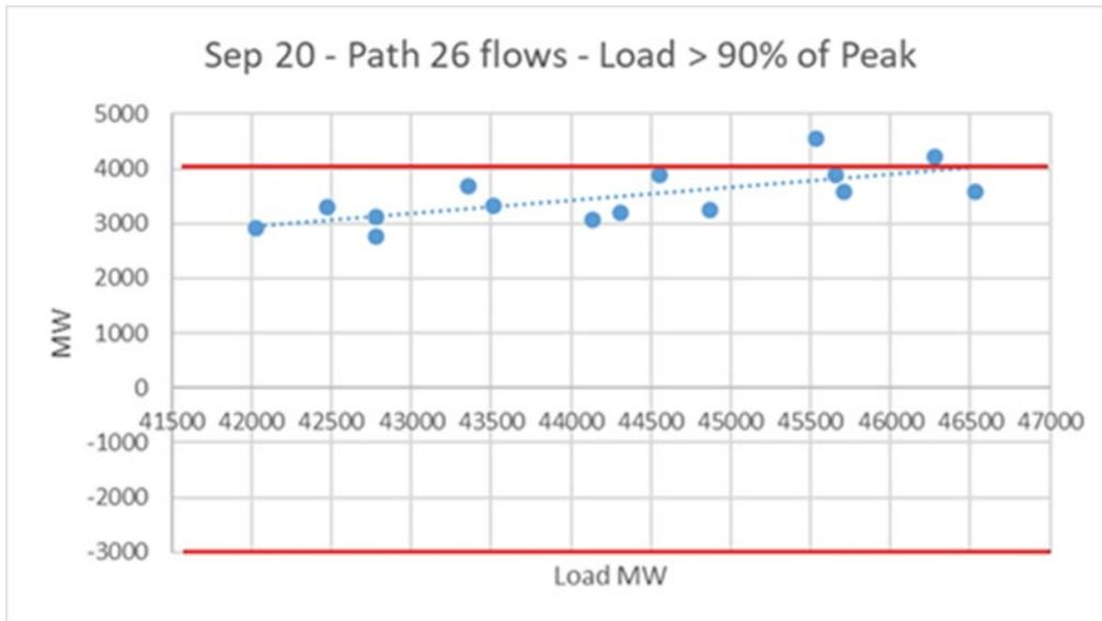
Graph 2: Path 26 loading levels during September 2020 periods when the load was above 90% of the peak.
