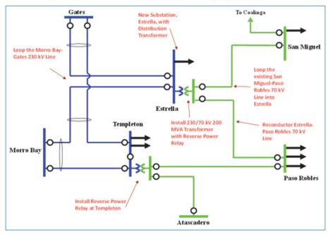
Figure 2: Paso Robles area after the Estrella project is in-service
