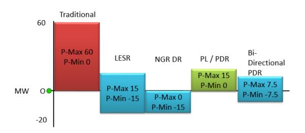
While referring to this element as a mid-point, it would not need to be symmetrical since a PDR might have more capability in one direction than the other (e.g. drop more load for supply since it could include processes and house loads while additional consumption might be limited to adding processing loads).
