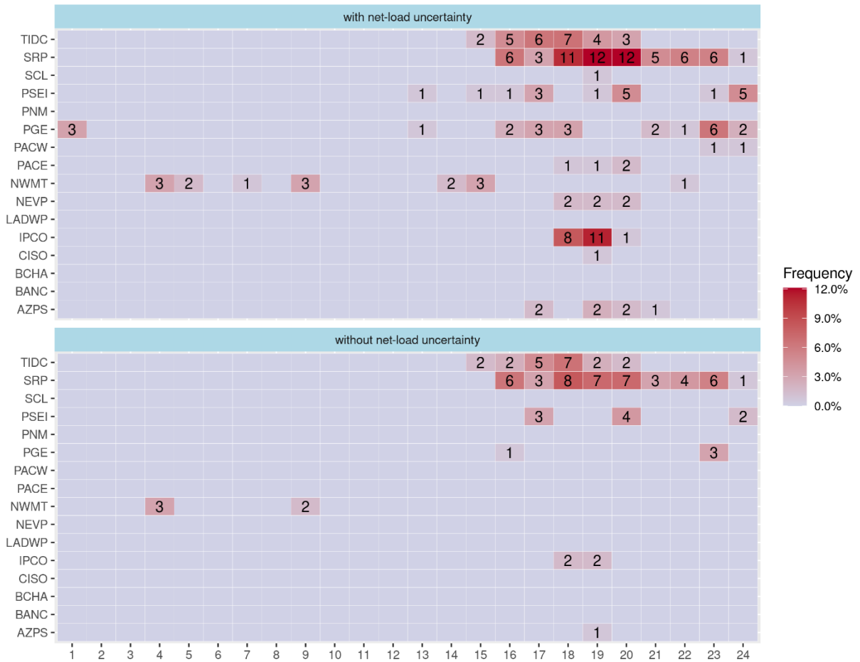
Figure 78: Daily Frequency of upward capacity test failures for all EIM BAAs
