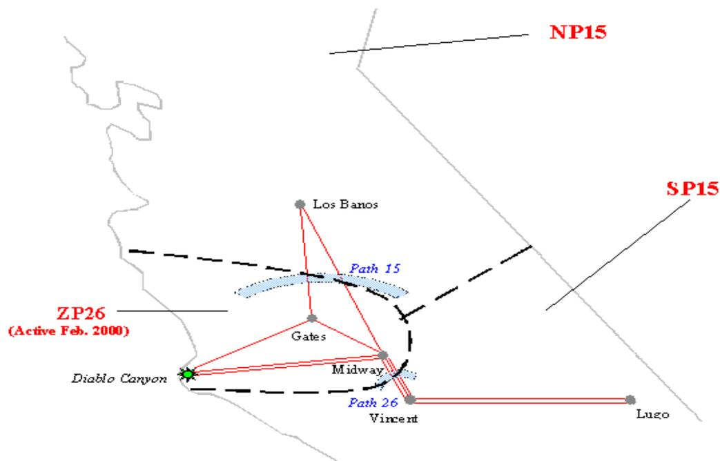
**We demonstrate the CAISO methodology by evaluating one of the proposed transmission upgrade options for Path 26. The upgrade being evaluated is the re-conductoring of the third 500 kV Midway-Vincent line.**
