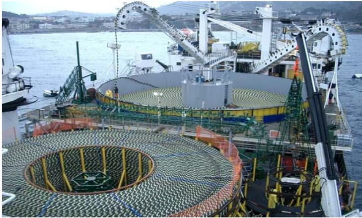
Barge (Shallow Water Cable Installer)
