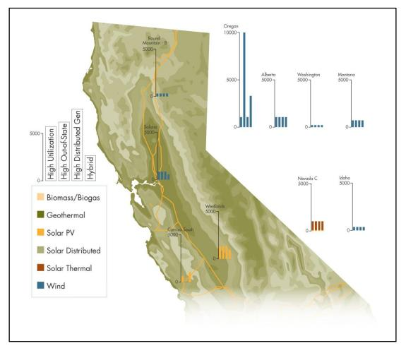
Fig. 5.1-5 Comparison of Energy Produced (GWh) from the Resources Selected in Each Scenario by Location and Technology in Northern California and Other Northern States
