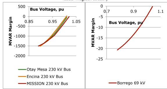
Figure 5.7-15 Q-V curves following Sunrise/SWPL N-2 contingency (portfolio 4 peak phase shifter and reactor mitigation solution)
