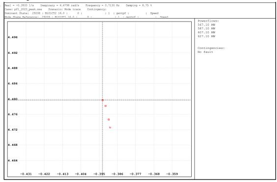
Figure 5.7-12 Mode trace scatters of CFE/SDGE mode as IID renewable increases
