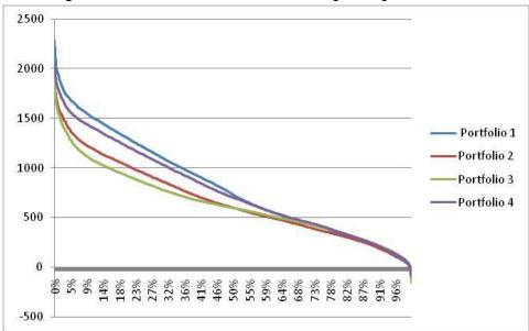
Fig. 5.8-7 Power flow duration curves of Pisgah-Lugo 500 kV lines
