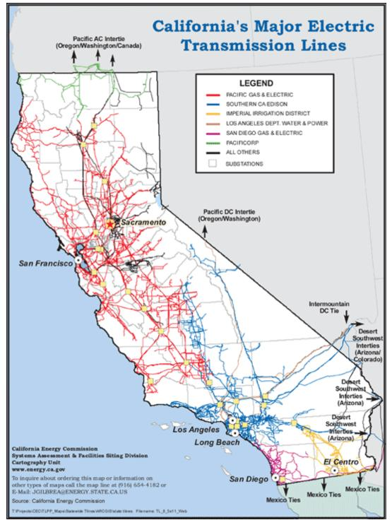
Figure 6.2-6: Overview of California Transmission System
