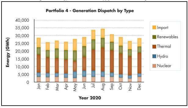
Figure 6.2-3: Types of Generation Supply to the California Region
