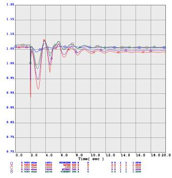
Figure 5.7-6 Bus voltages after NE/SE separation- portfolio 4 off-peak load
