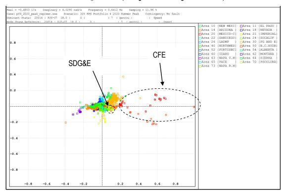
**Figure 5.7-19** Mode Shape Scatter of SDG&E Mode (0.786 Hz) following Sunrise/SWPL N-2 contingency (portfolio 4 peak generation mitigation solution)
