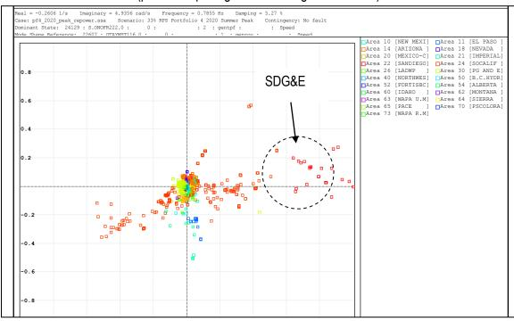
**Figure 5.7-20** Mode Shape Scatter of CFE Mode (0.567 Hz) following Sunrise/SWPL N-2 contingency (portfolio 4 peak phase shifter mitigation solution)
