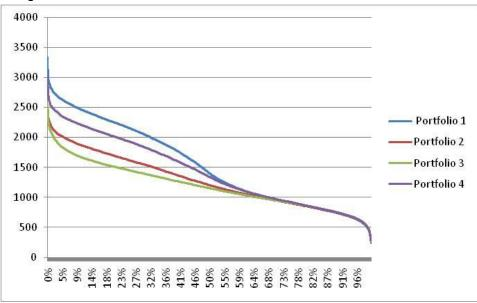
Fig. 5.8-8 Power flow duration curves of Colorado River–Devers 500 kV lines
