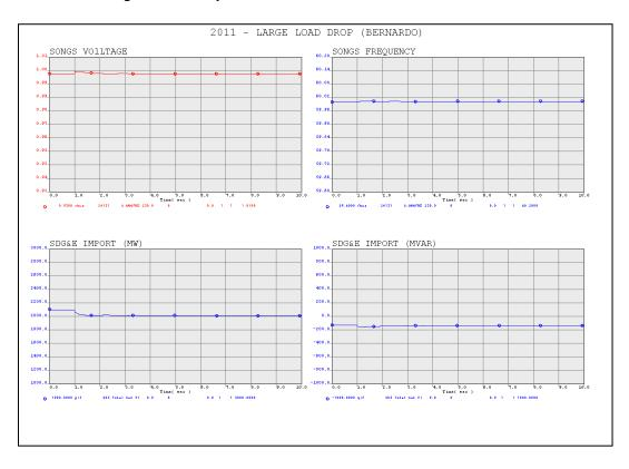
Figure 2.19-4: System Performance under Sudden Loss of Load
