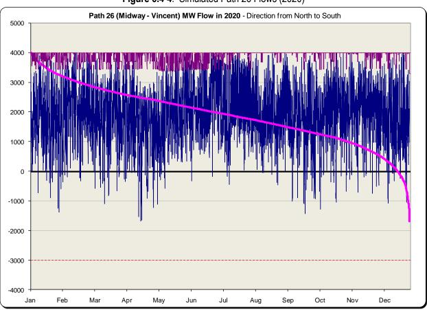
Figure 6.4-4: Simulated Path 26 Flows (2020)
