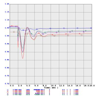
Figure 5.7-2 Bus voltages after NE/SE separation- portfolio 1 peak load
