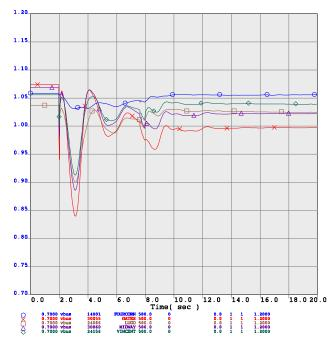
Figure 5.7-4 Bus voltages after NE/SE separation- portfolio 4 peak load
