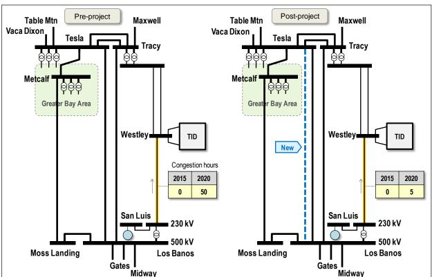
**Figure 6.4-8**: Congestion Mitigation for LBN – Alternative 1: Build a New Los Banos – Tesla 500 kV Line #2
