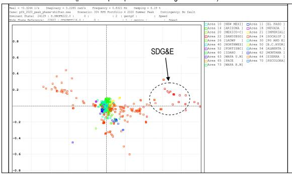
Figure 5.7-22 Mode Shape Scatter of CFE and SDG&E (0.648 Hz) Mode following Sunrise/SWPL N-2 contingency (portfolio 4 peak phase shifter and reactor mitigation solution)
