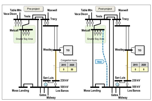
**Figure 6.4-11**: Congestion Mitigation for LBN – Alternative 4: Build a New Los Banos – Metcalf 500 kV Line
