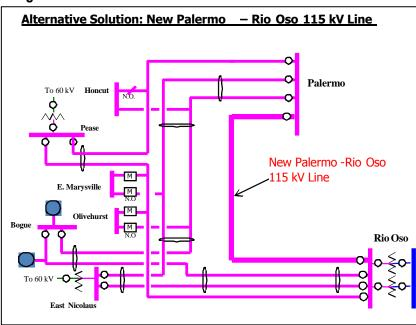
Figure 2.7-7: Alternative Solution - New Palermo-Rio Oso 115 kV Line
