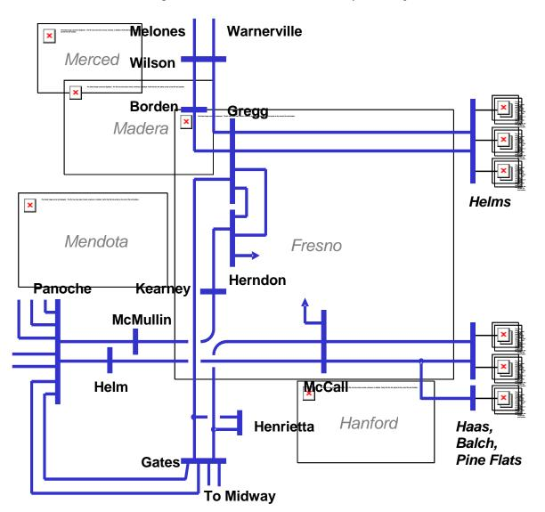
Fig. 5.6-10 Fresno area transmisson system diagram
