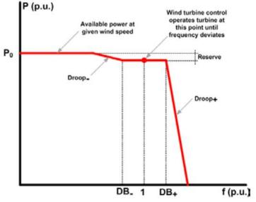
Depending on the technology of the WTG this units could provide FFR/PFR without reserving Headroom, but with high dependency of wind speed.
