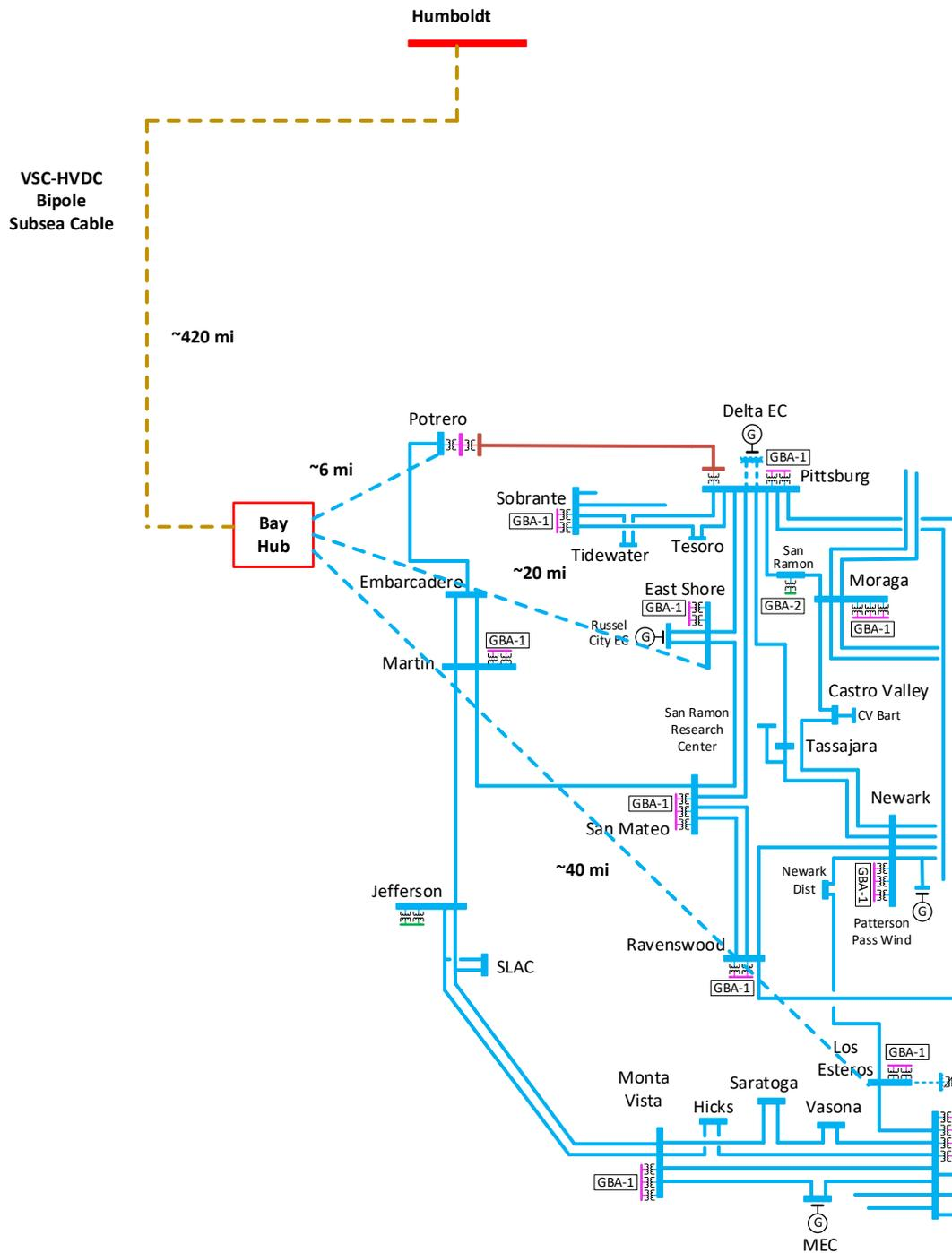
Option E: 500 kV AC Line to Fern Road and HVDC Line to Collinsville Initially Operated at 500 kV AC
