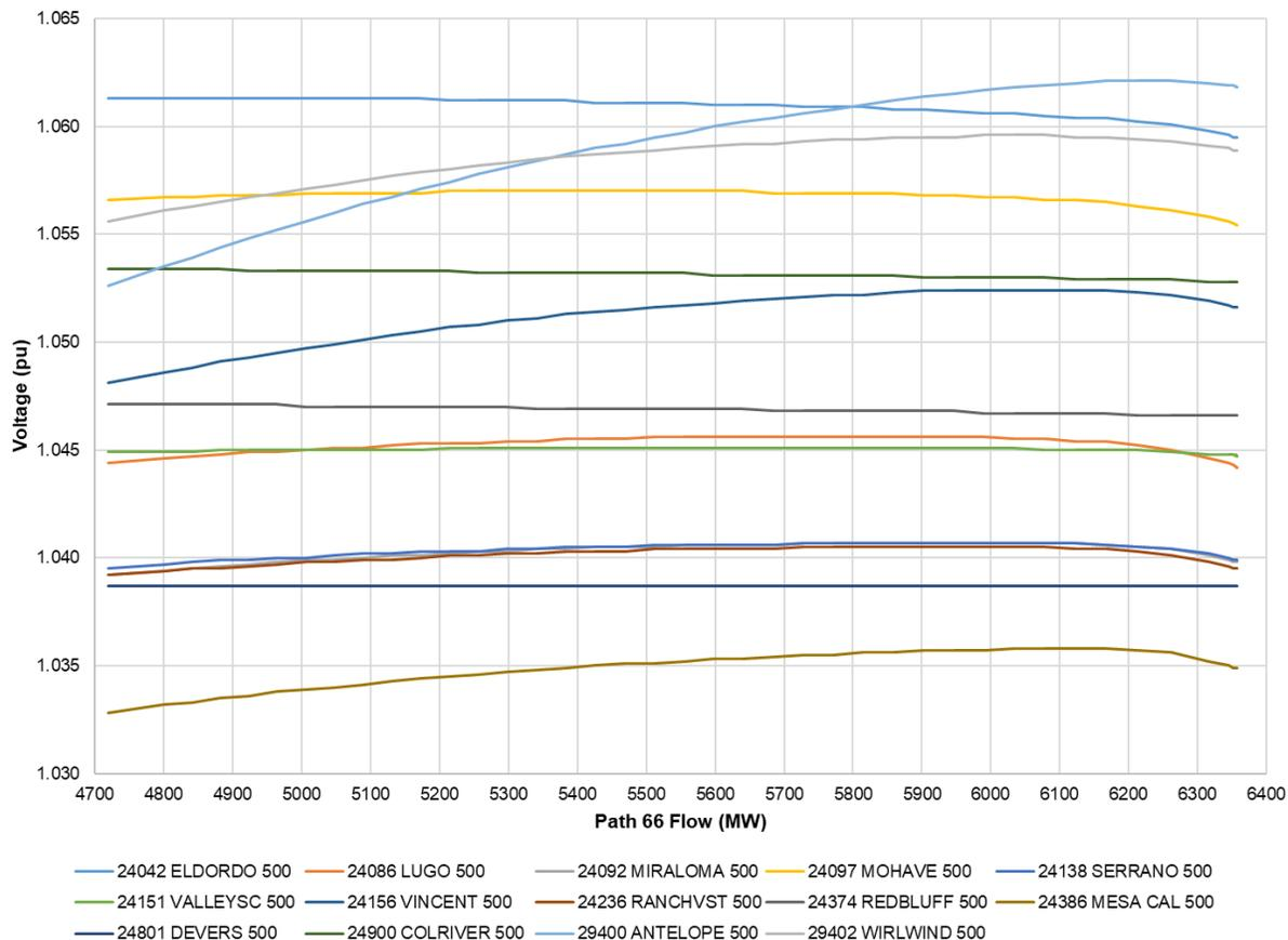
Figure F.11-3 displays that several of the northernmost 500 kV buses in PG&E system have a significant voltage deviation and the knee point of the PV curves occur with a post contingency N>S real power flow through Path 66 of around 6,350 MW, which is consistent with the results shown in Table F.11-8. Therefore, the swing bus generator exceeding its  $P_{max}$  limit in the post transient simulation is not the reason for the divergence and it is an actual steady state voltage stability issue.
