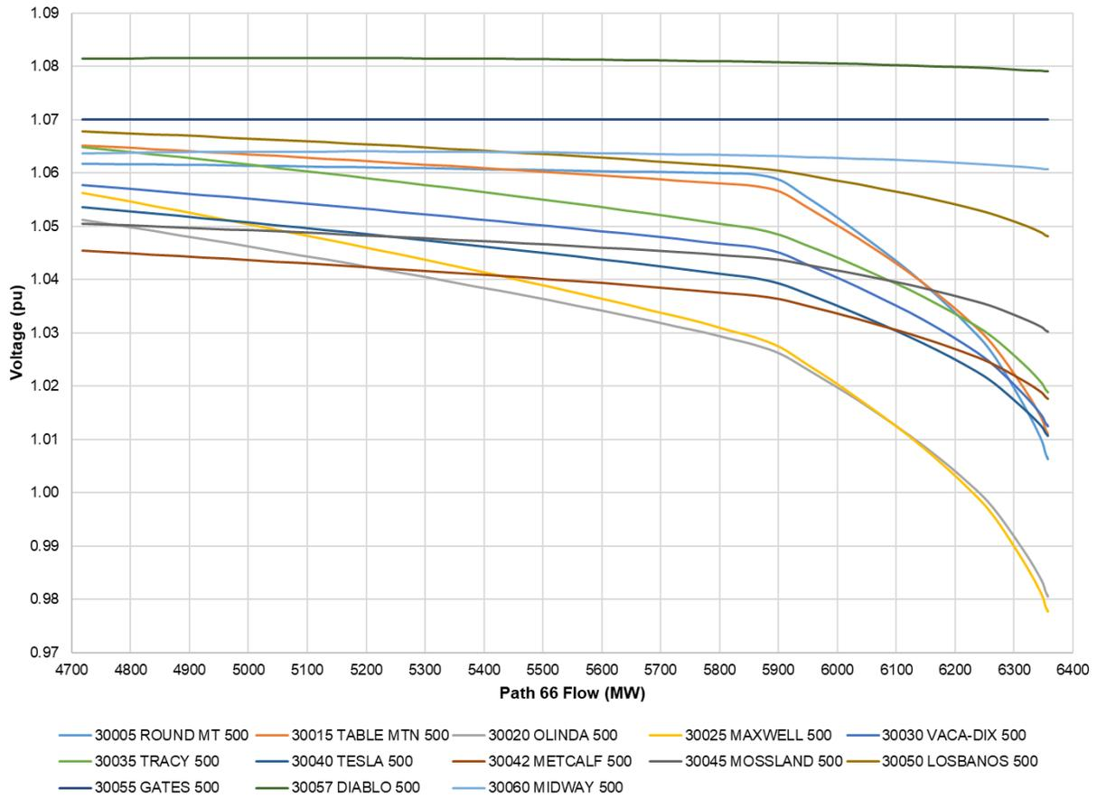
In a similar way, Figure F.11-4 illustrates the 500 kV voltages in Northwest area, where most of them exhibit a high voltage deviation near the knee point of the PV curve.
