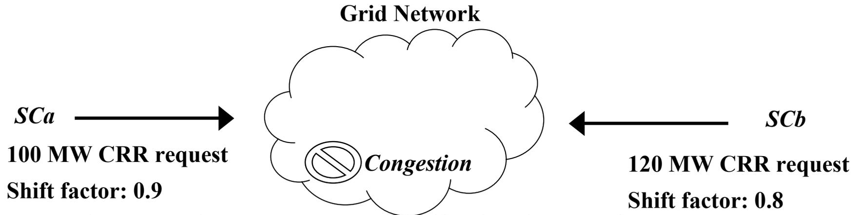
Assume the ISO has a constraint limited to only 96MW
