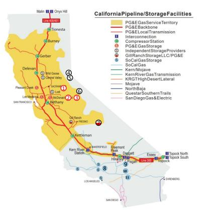
California Gas System Map from <a href="https://www.pge.com/pipeline/en.html">https://www.pge.com/pipeline/en.html</a>
