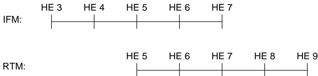
In this example, a short start resource is ISO-committed in the IFM for hours ending 3-7, and is subsequently committed by the ISO in the RTM for hours ending 5-9. If the resource's meter data show that it meets its Pmin at any point during hours ending 5-9, then its entire qualified start-up costs will be included as costs in the day-ahead BCR calculation.
