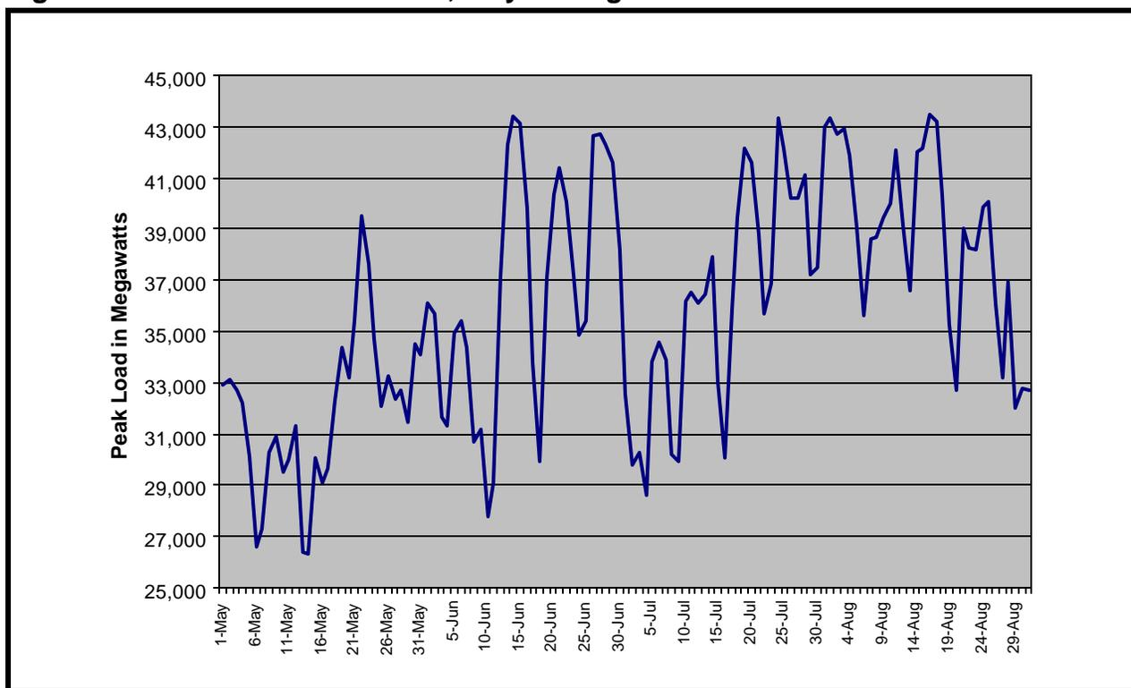
Turning to the Cal-ISO area, Figure 2-6 shows daily peak-hour load from May to August 2000. As the figure shows, peak load is volatile over a fairly wide range, sometimes swinging rapidly from under 30,000 MW to over 40,000 MW. Managing these fluctuations is a complex task under any circumstance, but it becomes even more difficult in a complex market environment in transition. Forecasting load then becomes particularly important for maintaining the reliability of the system.
