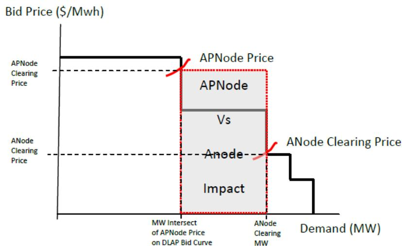
**Figure 6: Illustration of APNode and ANode difference Impact**
