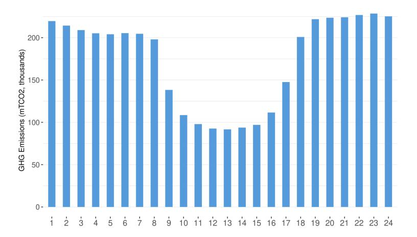
The above figure reflects the hourly sum of GHG emissions from internal ISO dispatches and GHG emissions from imports serving ISO load for the month of October 2024.
