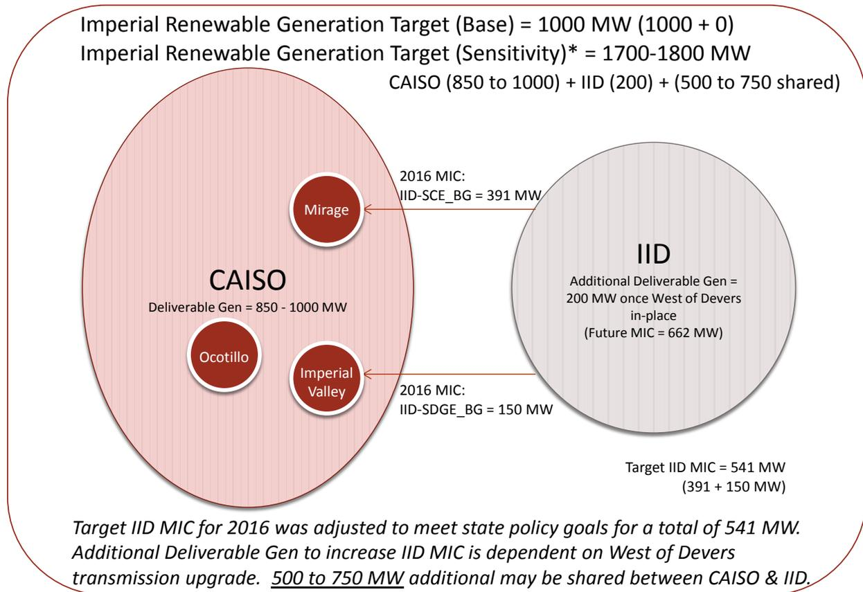
CAISO’s explanation of its last 3 years of deliverability assessments highlights that the methodology does not align deliverability allocation between CAISO and IID interconnections based on the actual physical constraints of the two interconnected systems.
