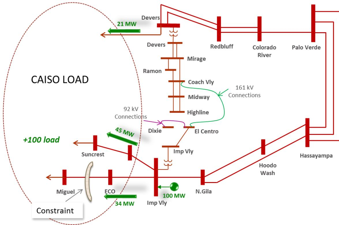
Figure 7. Impact of 100 MW Generator Interconnected at Coachella Valley Substation on ECO-Miguel 500 kV Constraint
