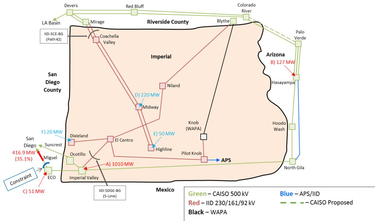
**Figure 9. Flow Impact of IID Interconnected Generators**
