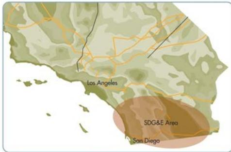
The SDG&E system, includes its main 500/230 kV and 138/69 kV sub-transmission systems. The geographical location of the area is shown in the adjacent illustration. Its 500 kV system consists of the Southwest Powerlink (SWPL) and Sunrise Powerlink (SRPL) systems. The 230 kV transmission lines form an outer loop located along the Pacific coast and around downtown San Diego with an underlying 138 kV and 69 kV sub-transmission system. Rural
