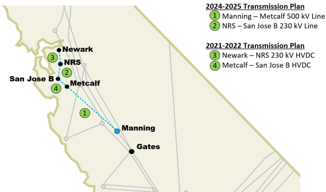
Figure 1. Recent Transmission Projects driven by large load forecast increases. Projects (3) and (4) were modified in November 2024 to provide increased capacity to the area and better position the system for additional expansion. Project (3) was converted to an AC solution at that time.
