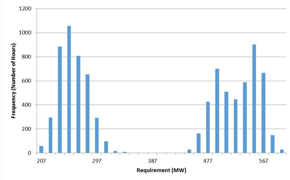
The annual (8,784 hours) average of regulation-up requirement by hour (see Figure 2) shows a pattern that the regulation requirement is more in proportion to load value than to the minute-by-minute variations of net load. The CAISO’s methodology uses net load, as opposed to gross load, in calculating regulation and load following requirements. It is not clear the extent to which the differences materially impact the production costs and the integration adder cost results.
