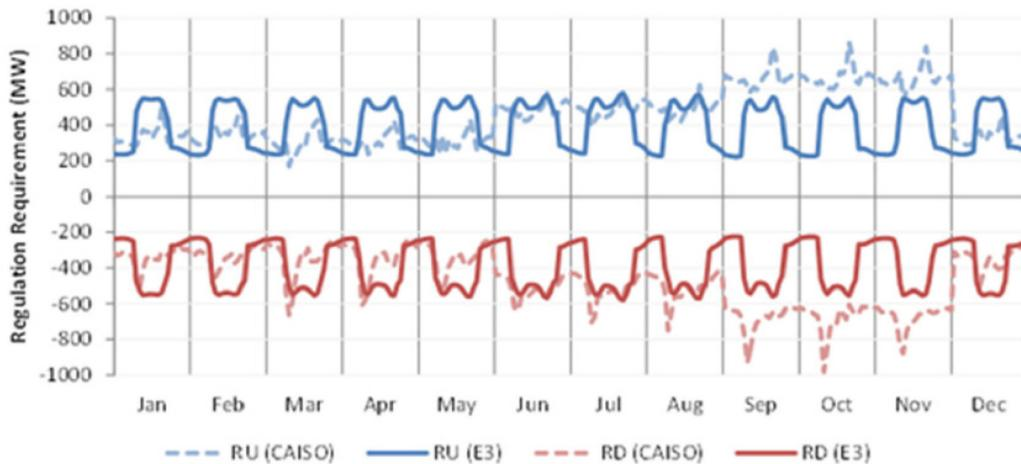
Lastly, the CAISO notes that the regulation and load-following input data indicate that the 1000 MW incremental solar PV seems to have no impact on regulation and load-following requirements. Case 2 and 6 have identical regulation and load-following requirements. Again this is counter intuitive to the expectation that changes in the amount of load-following and regulation would occur with changes in amount variable resources.
