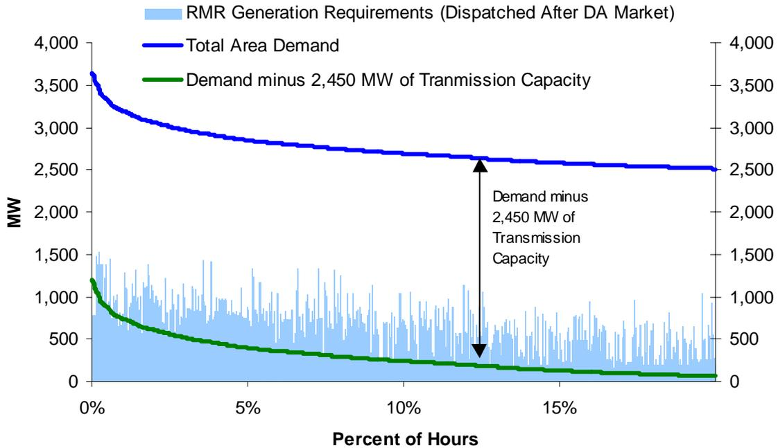
As shown in Figure 9, minimum generation requirements for RMR units issued after the Day Ahead market based on expected load conditions virtually always equal or exceed the amount of demand that would need to be met by generation inside the Basin under typical conditions, with 2,450 MW of transmission capacity available.
