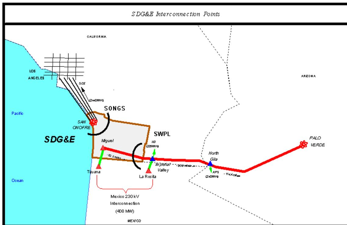
The non-simultaneous import capability used to represent a critical *N-1* contingency in Reliability Must-Run (RMR) planning studies and daily RMR dispatch decisions is 1,900 MW. The non-simultaneous import limit of 1,900 MW is based on the available capacity for importing power via the five 230 kV lines south of SONGS when the SWPL is out of service.
