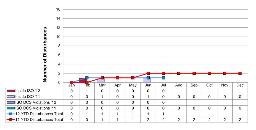
**Frequency Disturbances** are results of a sudden loss of load or generation.
