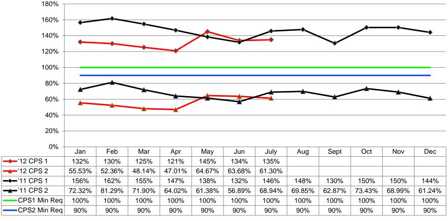
**CPS1** is a statistical measure of area control error (ACE) variability. It measures ACE in combination with the interconnection frequency. The CPS1 formula was developed on a conformance scale, therefore values over 100% are not only desired, but also expected. **CPS2** is a statistical measure of ACE magnitude. It is designed to limit a control area's unscheduled (or inadvertent) overflows that could result from large ACE values.
