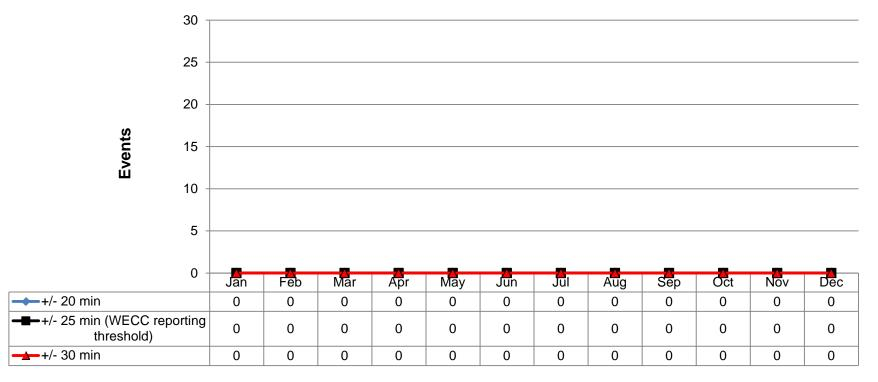
Reliability Based Control (RBC) is an Eastern and Western Field Trial that supports the Interconnection frequency by requiring balancing areas to take action to limit the duration of operating outside a variable area control error (ACE) bound that gets "tighter" as actual frequency deviates further from 60 Hz., during field trial reporting, which is required, but not considered a violation. The following actions are taken when exceeding balancing area ace limit (BAAL) -- high or low for:
