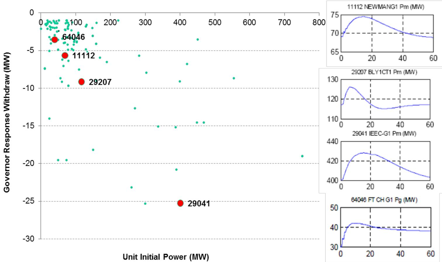
“Withdrawal” - any machine that is producing less power at 60 seconds than it did at any point earlier in the simulation
