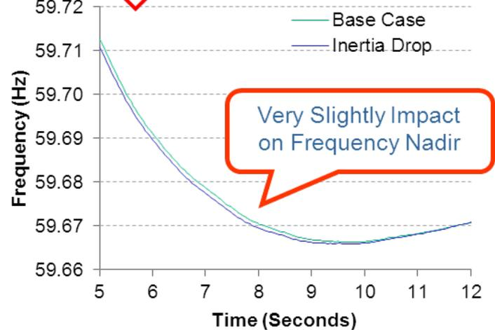
The impact of loss of inertia for 1993 MW is nearly invisible.
