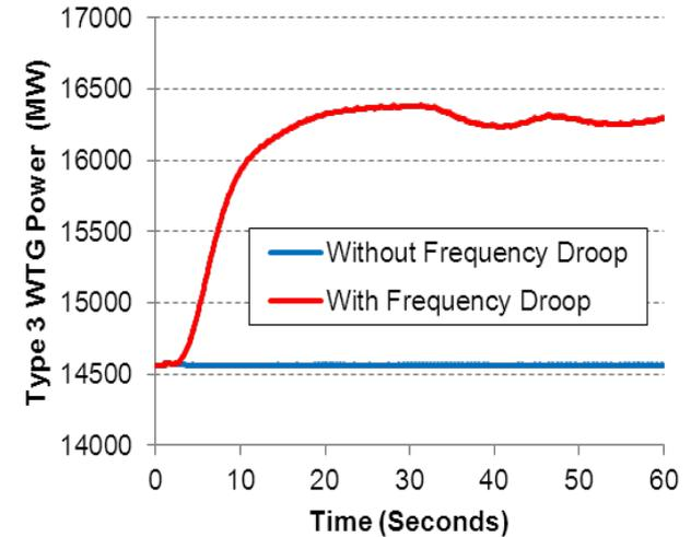
Primary frequency response from wind generation has the potential to greatly improve system frequency performance of the entire WECC grid.
