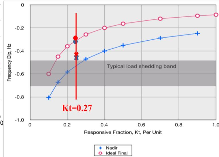
Load control has relatively small impact on the frequency nadir.
