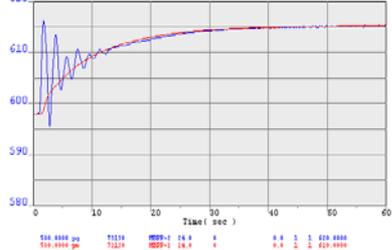
dPgen (Blue) and dPmech (Red) of Revelstoke Unit (MW) -DACE
