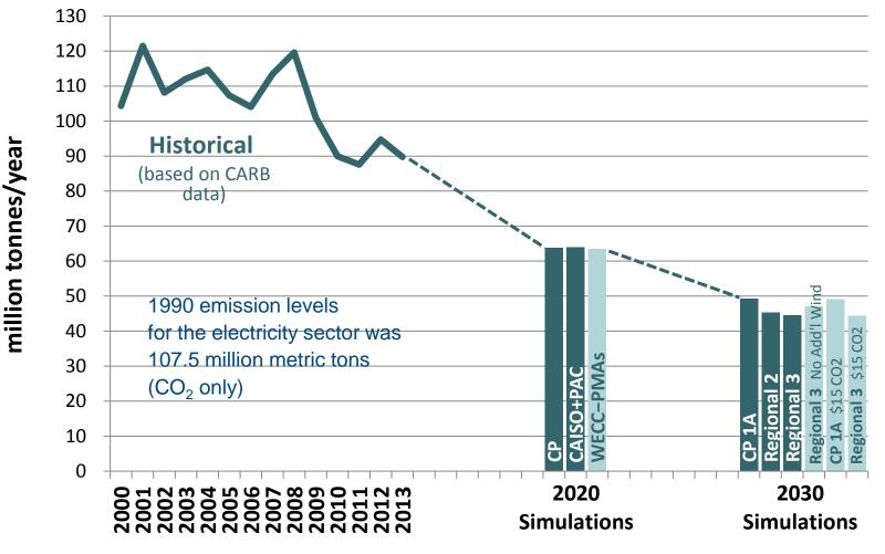
\* Simulation results assume CO<sub>2</sub> emissions associated with <u>imports are charged</u> and <u>exports are credited</u> based on a generic CO<sub>2</sub> emission rate for natural gas CCs.
