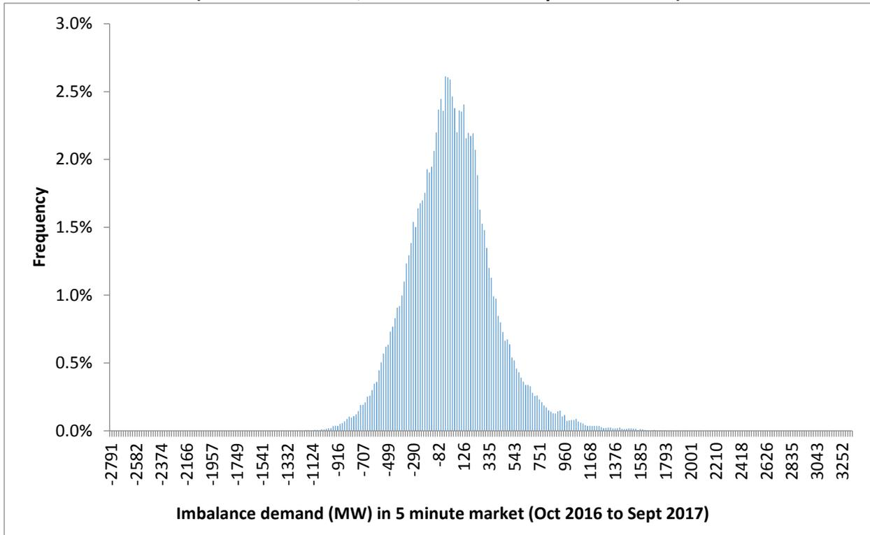
**Figure 4. Imbalance energy demand compared to total load for the APS BAA
