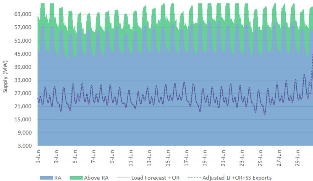
Figure 34: Supply capacity available relative to net load forecast in the day-ahead market
