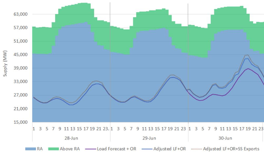
Figure 36: Supply capacity available relative to net load forecast in the day-ahead market – June 28-30
