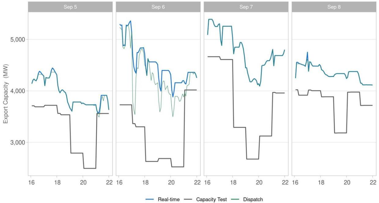
Figure 102: Supply capacity comparison test vs. RTM for Hydro
