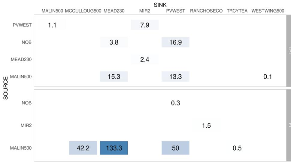
Figure 75: HASP maximum hourly volume (MW) of wheels by path in September
