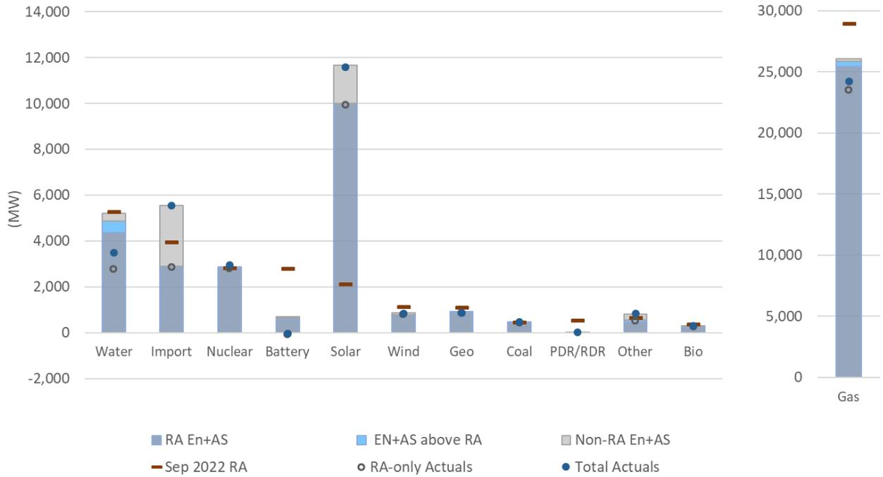
Figure 140: September 7 net peak (6:50pm). Real-time supply and actual production vs RA capacity
