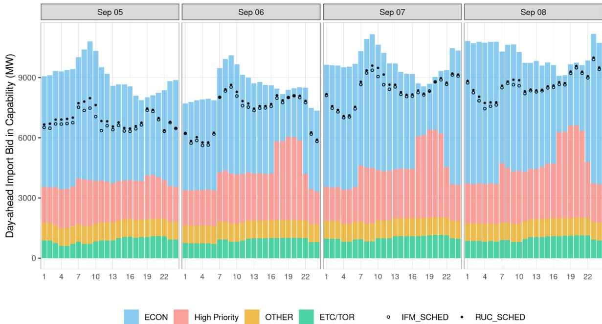
Figure 116: shows the RUC intertie schedules by schedule type. It also shows the overall net schedules as indicated by a solid black line. The net intertie schedules provide a more holistic reference of the supply available to the system once exports are balanced out with imports. The net intertie schedules reached their lowest levels in the early afternoon due to the large export volume cleared. The net intertie imports
