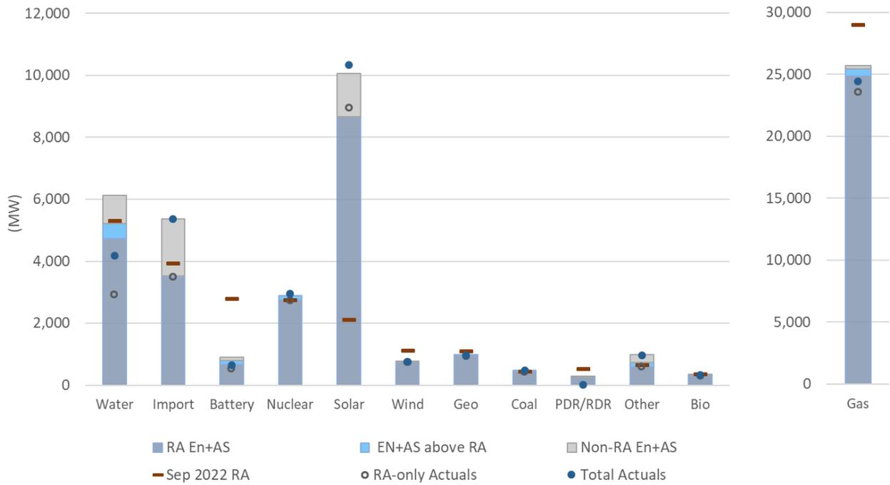
Figure 138: September 6 Net peak (6:58pm). Real-time supply and actual production vs RA capacity
