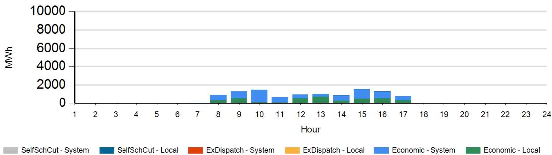
**2. Maximum wind/solar generation curtailment in MW for any one of the twelve real-time dispatch intervals in a particular hour.**
