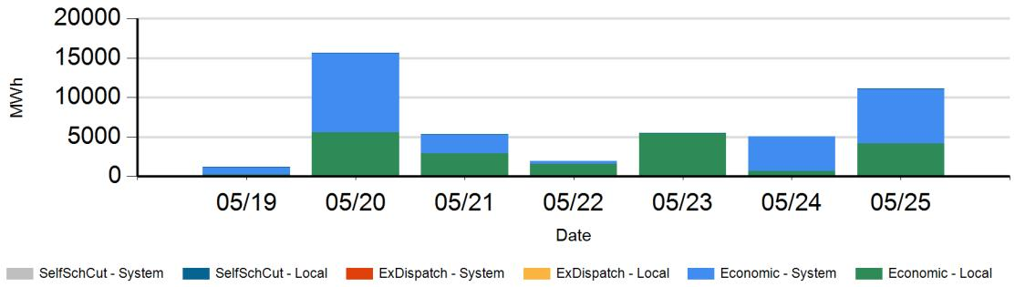
**4. Maximum generation curtailment in MW for any one of the twelve real-time dispatch intervals in a particular day on a 7-day rolling basis.**
